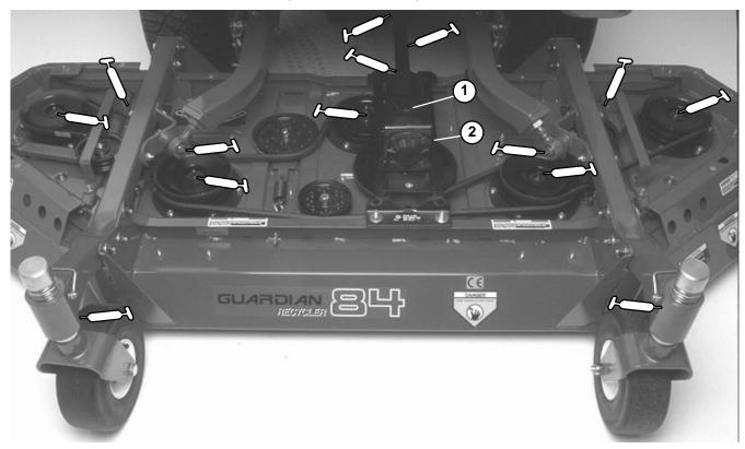
Figure 11 1. Filler Plug 2. Check/Drain Plug
